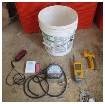
Paying proper attention to the 7 brooding basics requires making proper use of just 6 basic tools. Five of these, shown below the bucket, left to right, are relatively low-cost instruments that every grower should be familiar with: wind meters, smoke emitters, pressure gauges, air temp and humidity meters, and infrared temperature guns.
